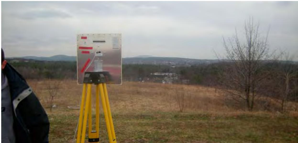
Our first stop, the nearest point (1500 ft), was very similar to the first test--full signal strength on the meter and crystal clear, low delay audio. The jitter buffers on our codec stats showed around 30mS buffering on each end, which is quite low. We could carry on conversations over the link easily.
