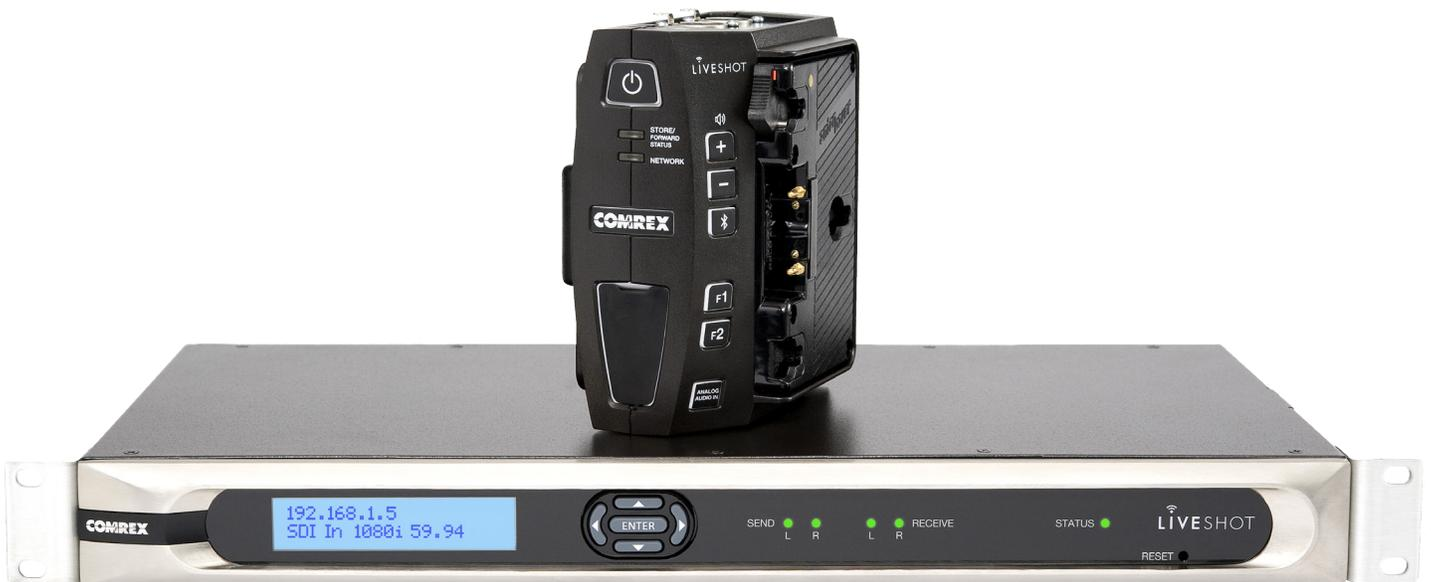
**1) Set up Comrex LiveShot Rackmount on a wired network that has port UDP 9001 open from the Internet.**
