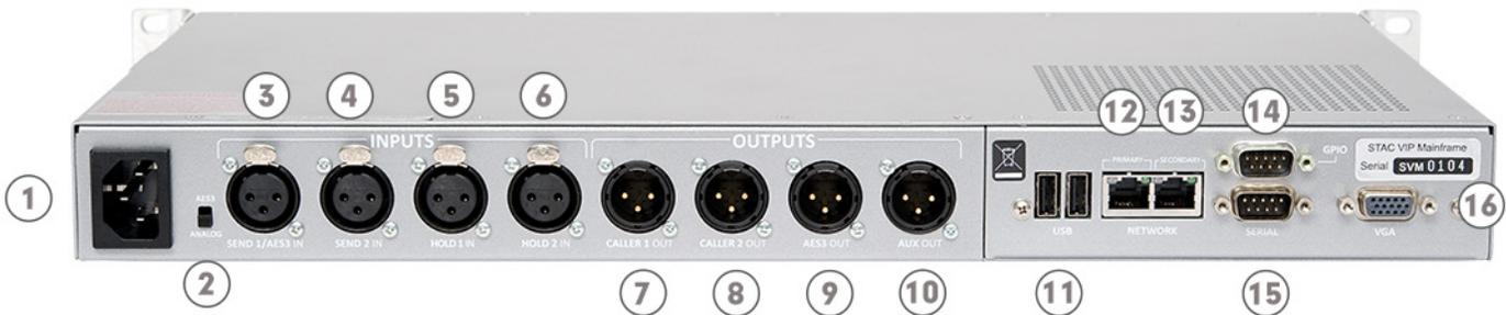
1) **Mains Power** - Apply universal mains power (110-240VAC) to the IEC connector here.
