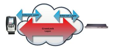
difficult to recover. In some modes, CrossLock can also signal encoders to "throttle down" their data rate to avoid congestion, reducing quality but maintaining reliability. CrossLock does this by building extra data streams between the codecs that relay important information (e.g. decoder statistics back to the encoder).
