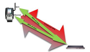
If you have multiple networks that are assumed good and have plenty of unmetered bandwidth, CrossLock can be set for Redundancy mode, whereby it will deliver the entire stream to each network. This can result in more of a guarantee of a seamless fallover if one network should fail completely.
