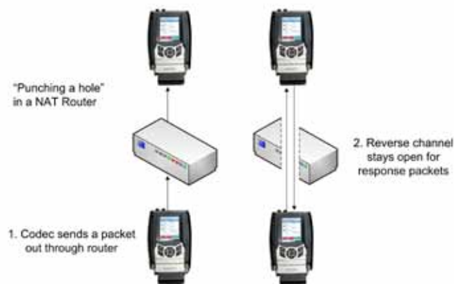
Figure 41 - “Punching a Hole” in a NAT Router
