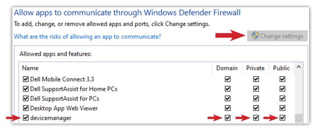
If Comrex Device Manager is already running, close the program and re-open it. As long as the computer in use is on the same network as Comrex devices, they should now be discoverable when using the "Scan for Devices" button.
