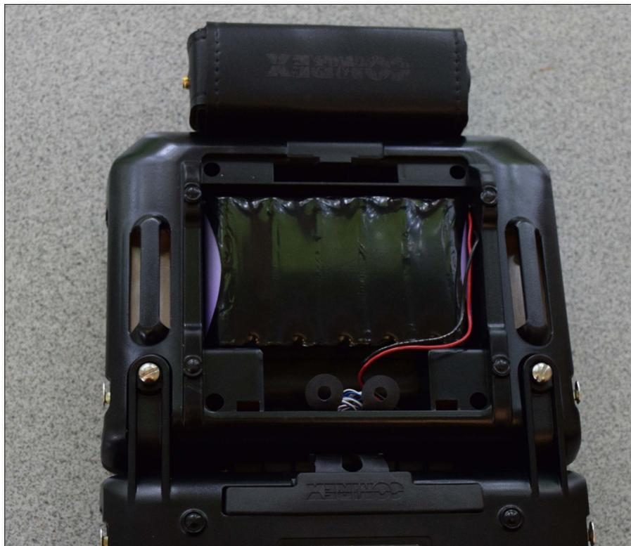
Attach the two rubber circles back to the battery compartment plate and place back onto the NX. Reattach hand strap. Insert rubber gasket into the groove on the mixer.
