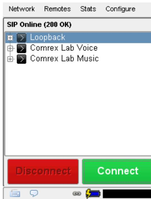
The status will reflect the progress of the registration process. When complete, this will display **Online**. If the box does not display Online after a short time, it usually means that registration attempt failed. It's best to go back and carefully check the registration info. It might also be useful to check that your registration information is valid by using it to configure a VoIP phone or softphone.
