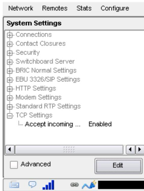
**Accept Incoming Connections** - Allows you to turn **TCP Auto Answer** on and off. Disabling this function means only outgoing TCP calls can be established.
