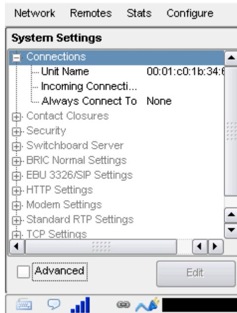
**Unit Name** - Users are encouraged to name their codecs here. The default name of a codec is the unique MAC address (Switchboard ID) of the Ethernet port. When this is changed to something familiar and unique (such as "Roving reporter", "Weather guy", etc.), the new name is reflected in several places:
