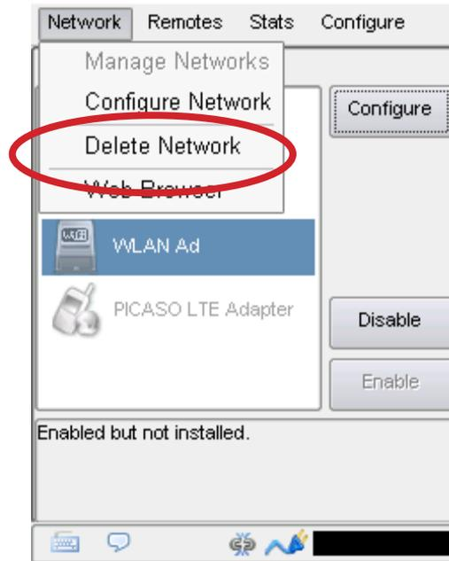
To delete a device, select it in the list (remember, it must be removed from the device), and navigate to **Network->Delete Network**.
