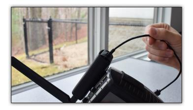
Run the supplied USB cable from the micro-USB socket on the Connect modem to the side USB connector on ACCESS.
