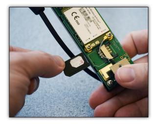
Once the SIM is installed correctly, reattach the modem's top cover and re-secure the thumbscrew.
