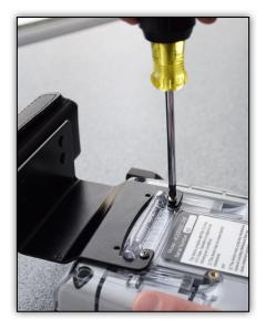
Align your standard Connect Modem bracket to the two top holes of the EXT bracket. Apply the two black screws with washers provided.
