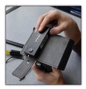
Fold the side flaps over the top of the modem on both sides.
