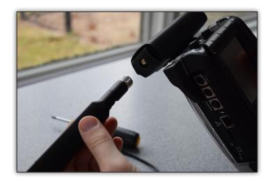
Connect the USB cable by seating the micro-USB into the micro-USB connector on the modem.
