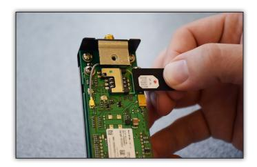
For the International Connect modem, the process is the same, but the SIM slot is in a different location.
