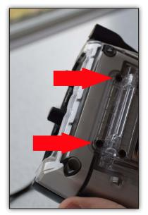
Place the pouch assembly so that the mounting screws align with these holes, and apply the provided mounting screws through both the pouch assembly and the handstrap slot assembly.
