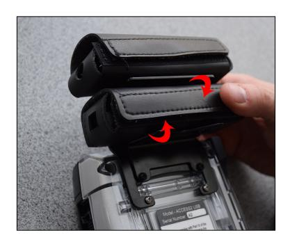
Repeat the steps for the top modem. Note that the circular and rectangular holes are opposite of the bottom modem.
