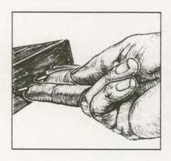
Before you set your program levels, raise the switches on the LXT/R to seize and extend. This must be done at both the remote and station end. Once the switches are raised, hang up the phone.
