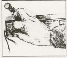
At the station end: The PEAK light on the LXT/R in the receive mode indicates that audio is being received at the correct level. When the light is flashing occasionally, the output of the LXT/R is around 0 dBu and should be able to feed most consoles without a problem.
