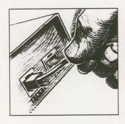
Plug the cord from the telephone into the TELSET SOCKET.
