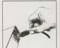
Plug the power cord (small end, without the converter box) into the POWER socket on the back panel. The big end goes into the wall outlet (120 vac).
