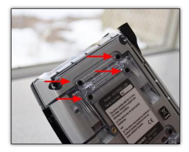
With the handstrap slot still attached and screws removed, take the EXT modem and align the 4 holes on the back plate to the four screw holes.
