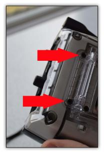
Place the pouch assembly so that the mounting screws align with these holes, and apply the provided mounting screws through both the pouch assembly and the handstrap slot assembly.
