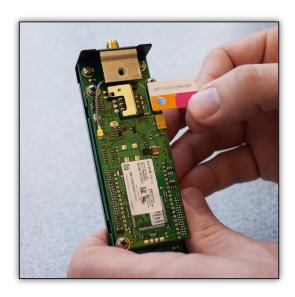
If using an adapter, first insert the SIM into the adapter as completely as possible, then apply the entire assembly to the SIM socket.
