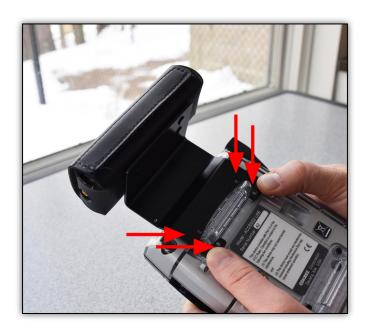
Apply the two silver screws provided with the EXT modem into the two bottom holes.
