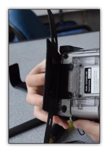
Align the modem in the pouch so that the SMA jack is lined up with the circular hole on the pouch and the micro-USB connector is aligned with the rectangular hole on the pouch.
