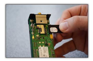
For the CJ and International Connect modem, the process is the same, but the SIM slot is in a different location.
