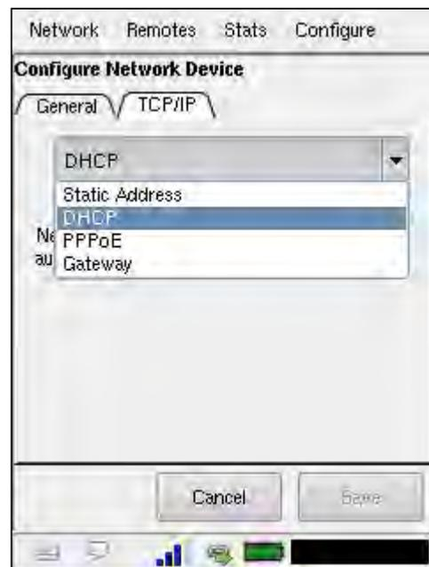
Figure 5 - TCP/IP Configuration
