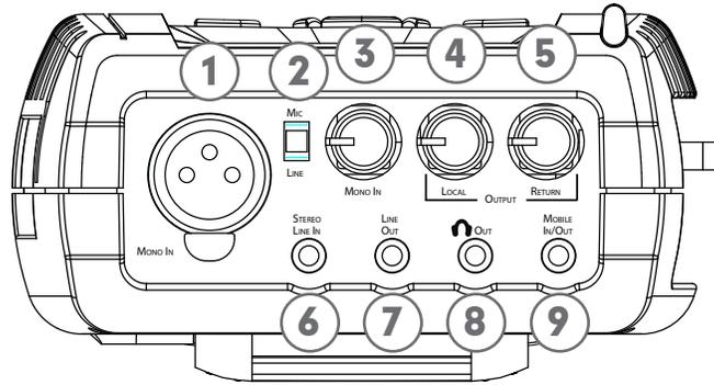
Figure 2 – Top Panel Diagram
