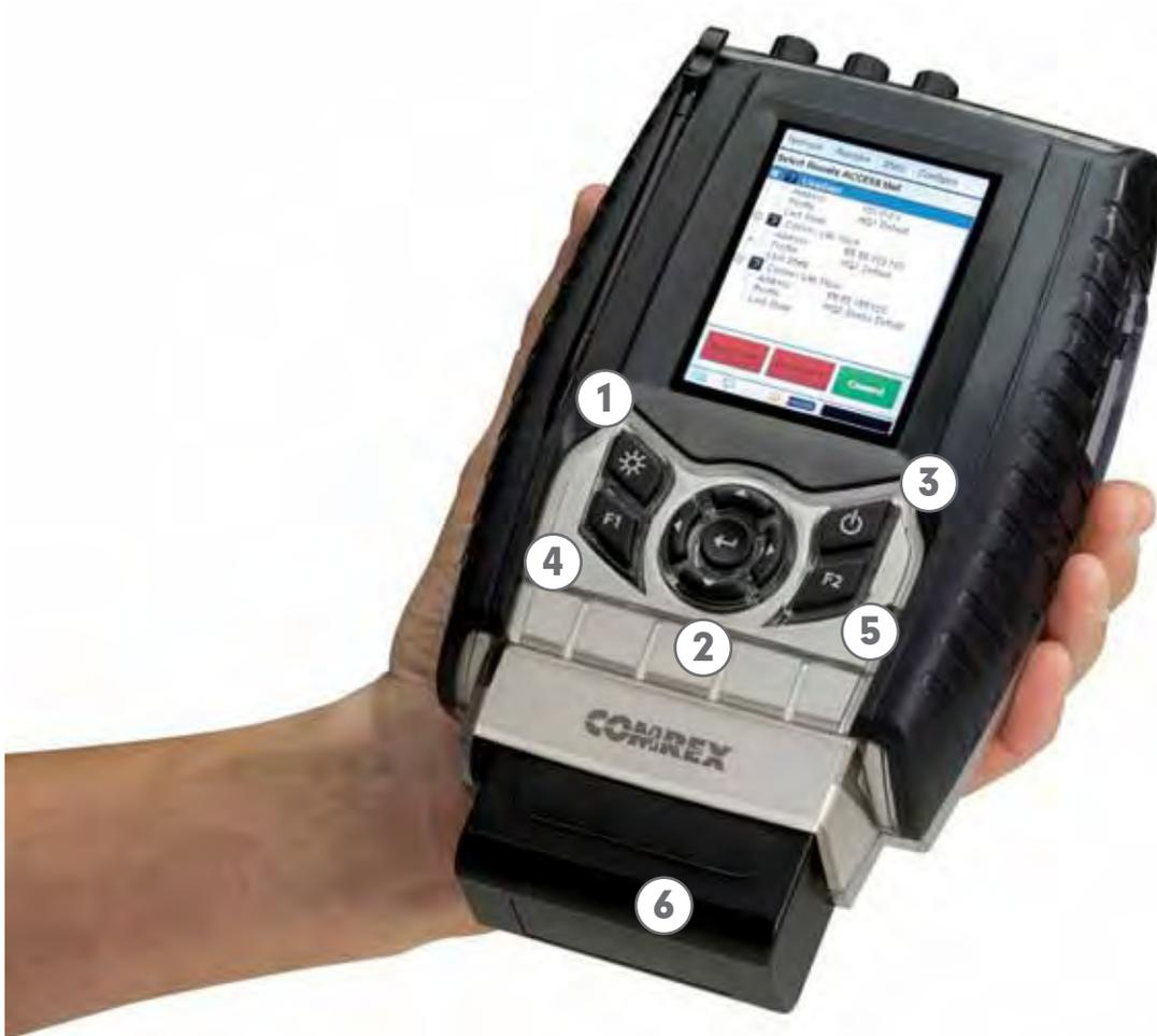
1) Backlight Key - Controls operation of the display light. Hold for one second to enable Power Saving Mode, where LCD lighting will turn off after ten seconds of non-use. Press the key to turn on light for another ten seconds. Hold for one second to enter Toggle Mode, where presses will turn light on/off. Hold for one second to return to default Always On Mode.
