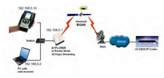
The ACCESS Portable, computer and BGAN terminal should be connected to a switch or directly with Ethernet cables, as shown in the diagram above. The computer's IP settings should be configured for DHCP. The ACCESS IP settings are described below.
