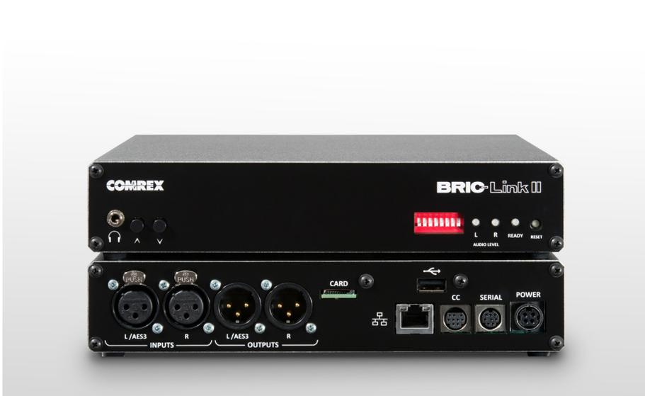
The Comrex BRIC-Link II, like the Comrex BRIC-Link, is a low-cost, high-performance solution for audio-to-IP conversion. Leveraging many of the core technical aspects of Comrex's successful remote broadcast ACCESS product line, BRIC-Link II provides for an elegant way of moving linear or compressed audio with very low delay.
