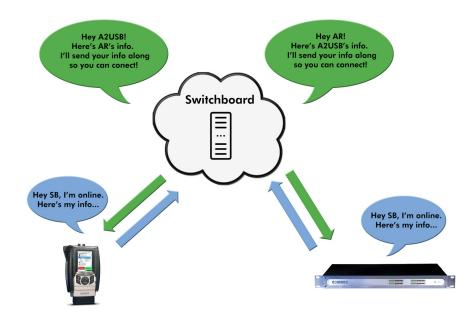
Switchboard allows for easy connections to be made between codecs without any knowledge of IP addresses on either end of the link. It also provides presence and status information about all the Comrex codecs in your fleet, and can help make some connections through routers and firewalls that might be difficult otherwise.
