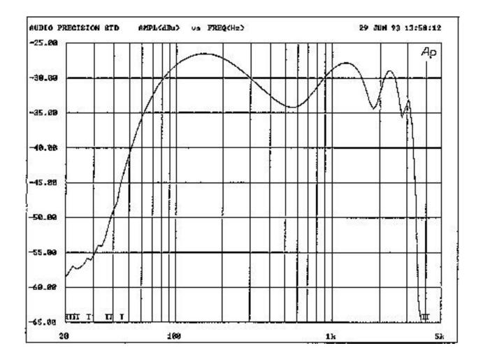
Curve 1 - Phone line with extension, before "Bridge Lifters" were installed. POTS
