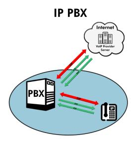
It's important to understand that the SIP protocol does not carry any actual voice between devices-- it simply instructs devices to create separate RTP sessions in each direction. RTP streams are created and destroyed based on commands contained in SIP messages when calls are made or received.
