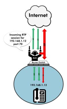
In reality, an ALG may often take quite a bit of license with your SIP connection. It can rewrite many of the SIP fields in order to comply with its rules, so the IP and port information getting to the service provider may actually be completely different than those sent by the device. As long as it has the intelligence to open the proper ports, this will usually work fine.
