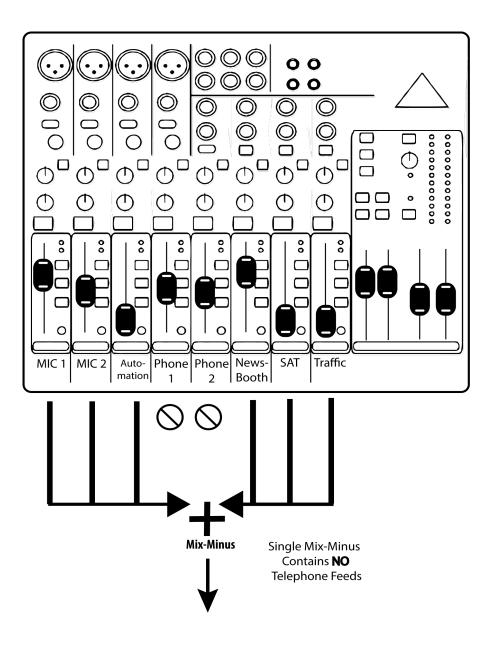
In some environments, it's only important that the caller hear the in-studio host, and less urgent that the on-air caller be able to hear automation, news reports, codecs etc. It's possible that simply routing an amplified version of the studio microphone signal to the "send" input will meet those needs.
