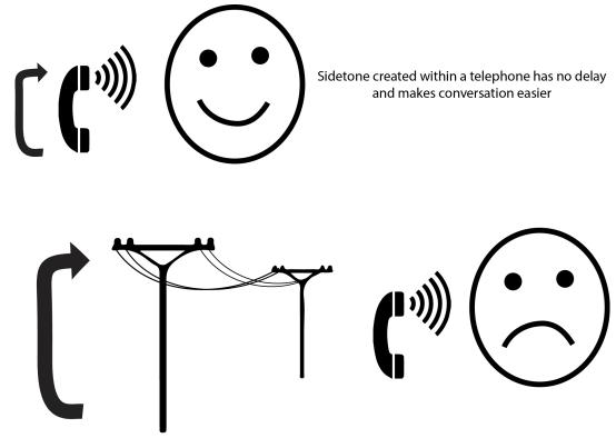
Sidetone created on the far end of a call has delay and makes conversation difficult
