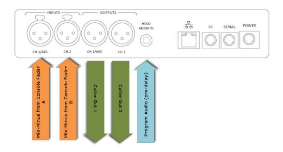
Finally, VH2 is capable of behaving like two, completely independent products for use in two, unrelated studios. This is shown below.
