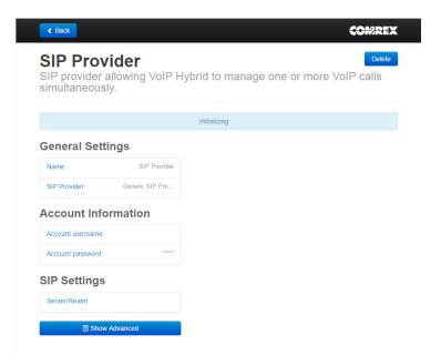
In Toolbox, navigate to **Channel Configuration->VoIP Providers->Add Provider-> SIP Provider**. The basic settings for a SIP provider are shown in the figure above. First, you should give your provider a unique name in the "**Name**" field. This is used for reference only.
