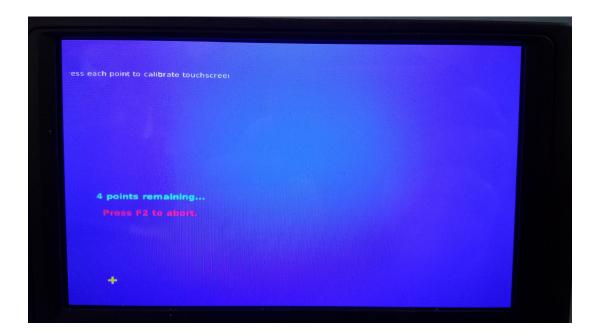
**4)** If your touch screen is unresponsive or uncalibrated, you'll need to reset the unit to factory defaults with the Device Manager utility. After that, the calibration menu will return on the next boot cycle and you can recalibrate your touchscreen.
