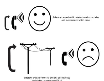
But for several reasons, sidetone is always generated locally within the speaker's equipment, rather than on the far end of the call. This is because humans have a very hard time handling even the smallest delay in this sidetone signal. In testing, we've found that any delay over 10 ms starts to create an effect called "slapback" where the speaker is unable to maintain conversation and begins to halt and stutter.
