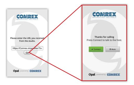
**Opal Connect** offers an experience nearly identical to users on browsers. The main difference is that **Opal Connect** does not offer a mic level meter. **Opal Connect** does not operate in "background mode" on mobile phones or tablets. If the app is running and sent to background (via "home" button or other means) the current call will disconnect. But since **Opal Connect** maintains and offers the last **Invite** when brought back up, it's a simple and quick reconnect process.
