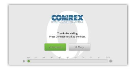
Pressing "Connect" will create a high quality audio link to one of the two Opal channels. The connection will end when the caller presses the "Disconnect" button.
