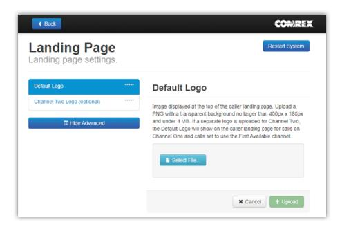
Choose the file to upload and then select "**Upload**" to send the graphic file to Opal. If a separate logo is uploaded for Channel Two, it will only be viewable on Channel Two. The Default Logo will show on the caller landing page for calls on Channel One. If a separate logo is not uploaded to Channel Two, the Default Logo will be applied on both channels.
