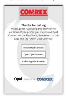
When **Opal Connect** is launched from a browser, the Invite will be shown in the URL bar of **Opal Connect**. If **Opal Connect** is launched independently from the browser, it will offer the last **Invite** used (if applicable) or a blank URL entry bar. It's possible to manually paste or enter an **Invite** into the URL bar. When the "**Go**" button is pressed, the app will display the Opal landing page.
