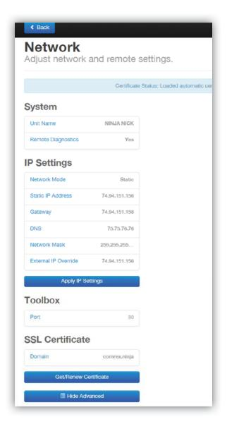
Change the mode to **Static**, and input the IP address, netmask, gateway and DNS information for your network. Click "**Apply IP Settings**" after all the information is correct. If you need to access **Toolbox** after this, you'll need to rescan and log in again (or open a browser to the new IP address).
