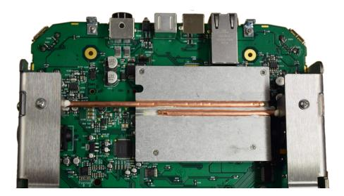
The metal plates on the sides of the unit are the natural place to vent this heat. The design is quite effective, keeping the CPU temperature below its throttling threshold even in the presence of 50°C (122°F) ambient temperature.
