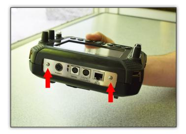
Place the bracket and pouch assembly so that the bracket mounting holes align with the top plate holes. Re-apply the two Philips screws. Proper installation of the single and dual modem brackets are shown in the photos below.
