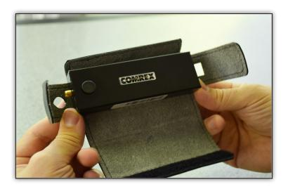
Fold the side flaps over the top of the modem on both sides.
