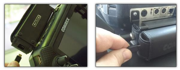
Run the supplied USB cable from the micro-USB socket of the NX Connect modem(s) to the respective side USB connector(s) on the NX.
