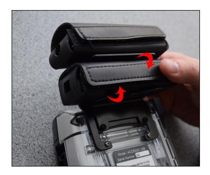
Repeat the steps for the top modem. Note that the circular and rectangular holes in the pouch are opposite of those in the bottom pouch.
