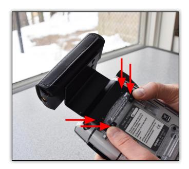
Apply the two silver screws (provided) into the two bottom holes.
