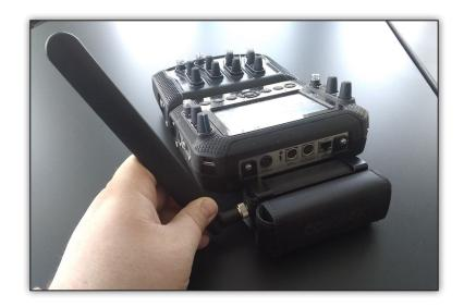
Connect the supplied USB cable by seating the micro-USB into the micro-USB connector on each modem as shown below.
