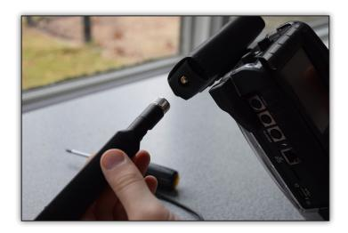
Connect the supplied USB cable by seating the micro-USB into the micro-USB connector on the modem.
