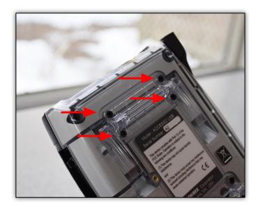
With the handstrap slot still in place, place the EXT bracket with pouch so the 4 holes on the bracket plate are aligned with the four screw holes of the handstrap slot.
