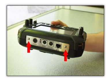
Place the pouch assembly so that the bracket mounting holes align with the top plate holes as shown below and on page 10. Re-apply the two Philips screws.
