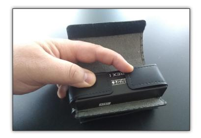
Fold the longer flap up and over the smaller flap attaching it to the velcro of the smaller flap. The pouch should be snug and securely closed. When using the Dual Pouch option, repeat this procedure for the second modem.
