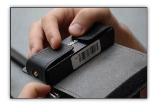
Lift the smaller flap on the back side of the ACCESS Portable so that the velcro is facing out along the back of the modem. Fold the longer flap with the Comrex logo over the modem and attach to the smaller velcro flap.
