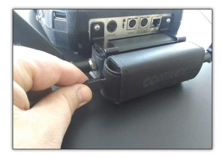
Run the USB cable from the micro-USB socket on each of the Comrex Connect Modems to the respective side USB connectors on the NX.
