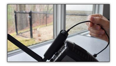
Run the USB cable from the micro-USB socket on the Connect modem to the side USB connector on ACCESS.
