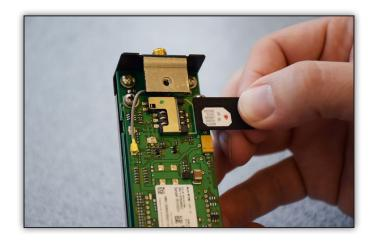
For the CJ and International Comrex Connect modems, the process is the same, but the SIM slot is in a different location.
