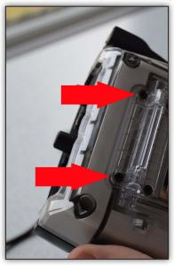
Place the bracket assembly so that the holes in the bracket align with the holes of the handstrap slot, and apply the provided mounting screws through both the bracket assembly and the handstrap slot.
