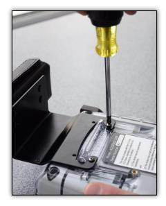
Align your standard Connect Modem bracket with pouch to the two top holes of the EXT bracket. Apply the two black screws with washers (provided).
