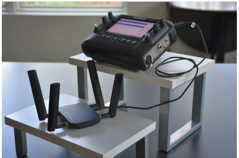
Pepwave modem connected to ACCESS NX
