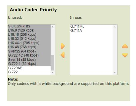
Using the Left Arrow in between the "Unused" and "In Use" lists, highlight and remove all codecs except for <u>G.711Mu</u> and <u>G.711A</u> as shown above. You are finished with the telephone setup.
