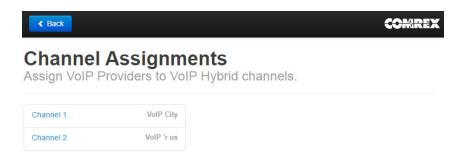
The figure shows each channel assigned to a different provider. Each channel could also be assigned to the same provider, and the usual behavior is for calls to "hunt" between the channels (first call on Channel 1, second on 2).
