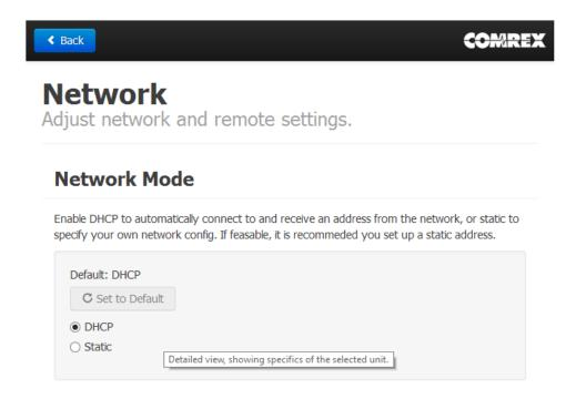
Change the mode to **Static**, and input the IP address, netmask, gateway and DNS information for your network. Click 'apply IP settings' after all the information is correct. If you need to access **Toolbox** after this, you'll need to rescan and log in again (or open a browser to the new IP address).
