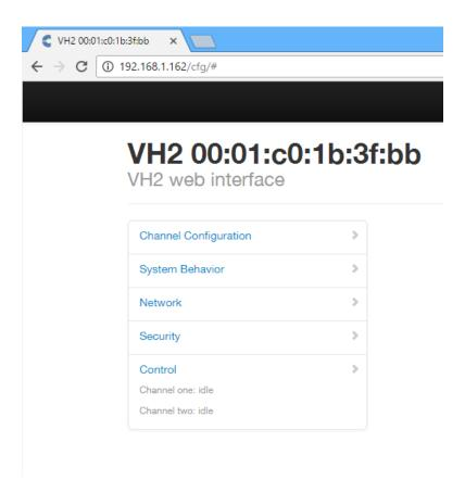
This menu gives you the ability to control each channel either by placing the calls on-air, on-hold, transferring to the handset or dropping the call. This allows you to control the VH2 channels without having to physically push the buttons.
