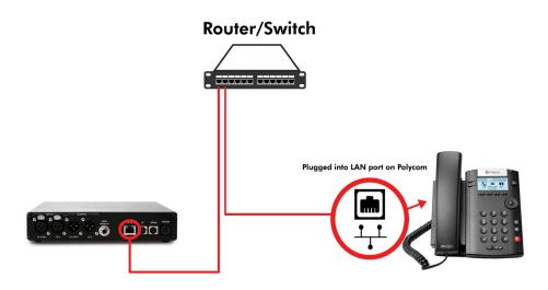
The second way is useful when you do not have two ports available. Plug the Polycom's ethernet port into the network. Plug the VH2 into the computer port (shown with a laptop icon) on the VH2. Both units will be treated as separate devices on the network.
