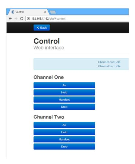
Additionally, it will show the status at the top of the screen for both channels.
