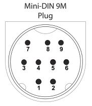
Contact closures are available via the 9-pin mini-DIN connector on the interface panel of the ACCESS Portable and BRIC-Link type units. Inputs are triggered by shorting the respective input to **Pin 9**. Outputs consist of an open collector circuit which will offer a high-impedance path to **Pin 9** when inactive, and a low impedance path to **Pin 9** when active. These outputs are capable of sinking up to 200mA at a voltage up to 12V.
